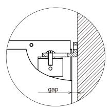
\* When you fix the basin body on the wall with no gap to the inclined wall, the basin body will be fixed improperly. It makes improperly between basin and basin body.
